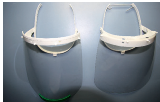
→ Fig. 2: Face shields with 3D-printed retainers
