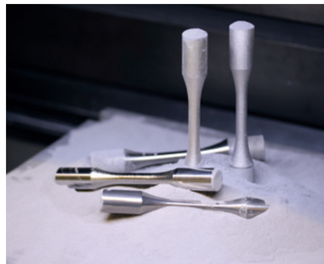
→ Fig. 3: Additively manufactured and post-processed specimens for the Additive Fatigue Study
