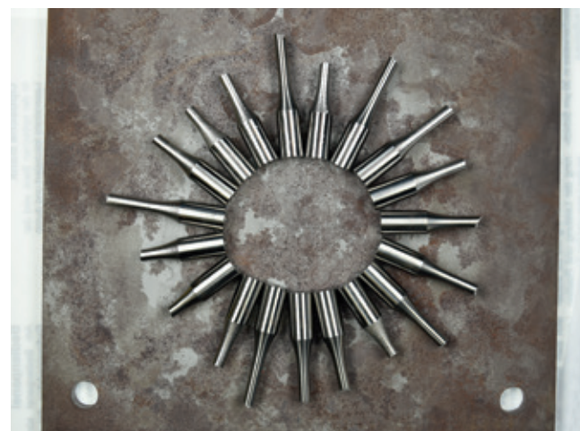
→ Fig. 4: Additive Fatigue Study specimens after testing
