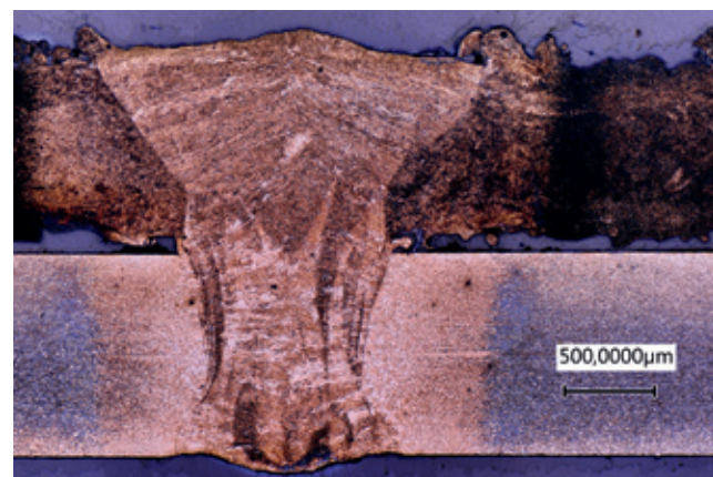
→ Fig. 1: Metallographic section of a laser welded joining specimen in the lap joint, printed LAM material above, rolled DP800 below
