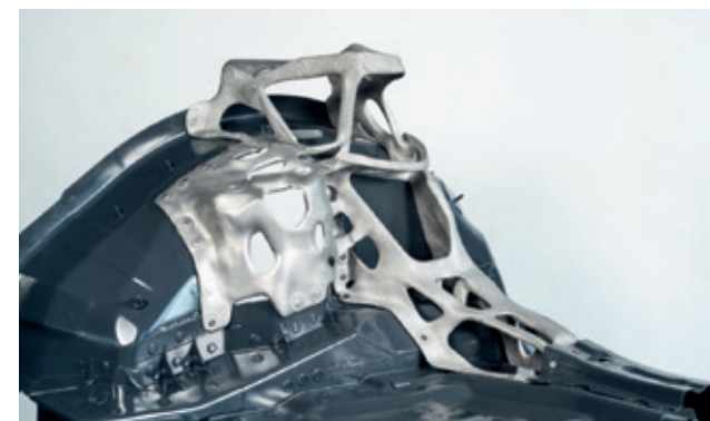
→ Fig. 4: Damper strut dome made of CustAlloy (EDAG)
