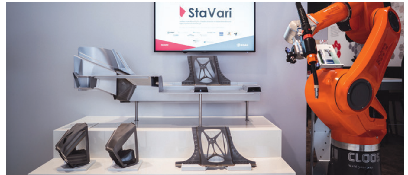
→ Fig. 2: Demonstrator assembly from EDAG designed for an EV that encompasses the wheel housing, additively manufactured C- and B-pillar nodes, rocker panel, and adjacent body side structure.
