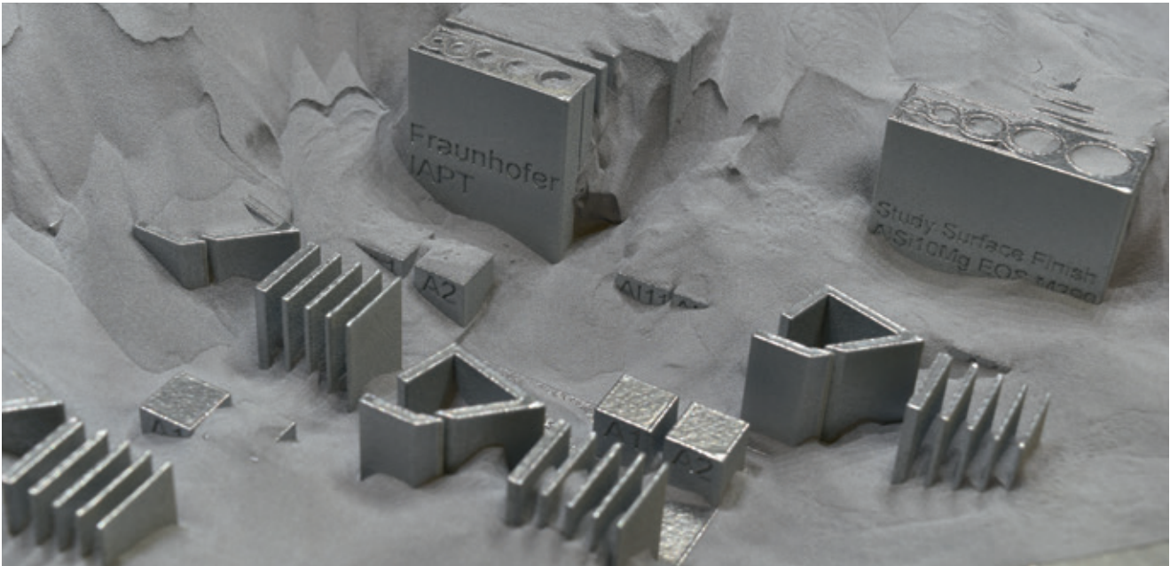
→ Fig. 1: Specimens for the Surface Benchmark Study
