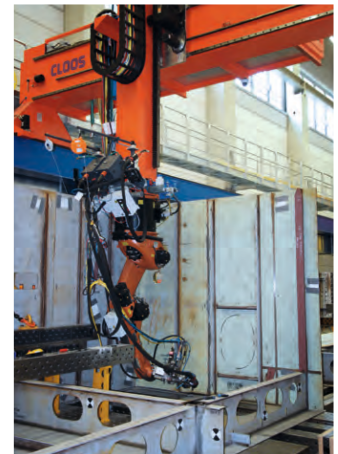
→ Fig. 2 and 3: 2) See photo above – ShipLight processing head from Cloos with integrated joint tracking sensors; 3) Fully automatic processing system in operation at Fraunhofer IAPT (source: Fraunhofer IAPT)
