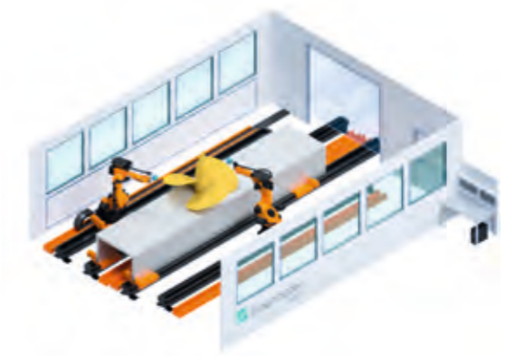
→ Fig.: Cell solution for stationary manufacturing of maritime components based on the WAAM process
