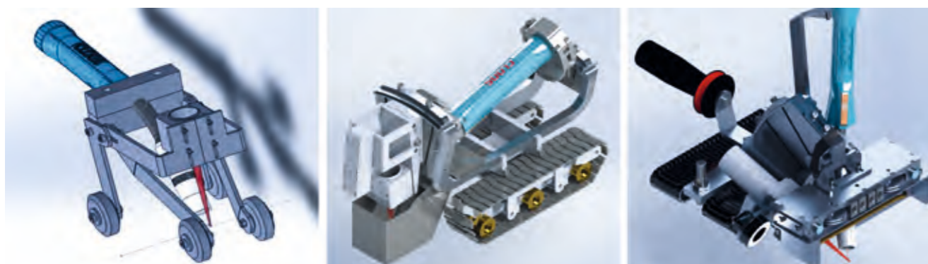
→ Fig. 4-6: Evolution stages of ShipLight manual welding unit for different joining layouts developed by Fraunhofer IAPT (Source: Fraunhofer IAPT)
