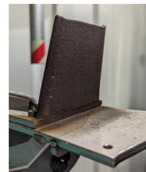
Layer-by-layer structure of the prong on the robotic arm of the Additive Mobile Factory®
