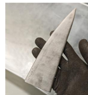
Prong for the mine clearance machine, printed using the cladding method
