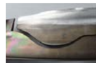
Reinforcement applied using DED (top), prototype of a reworked leading edge (bottom)
