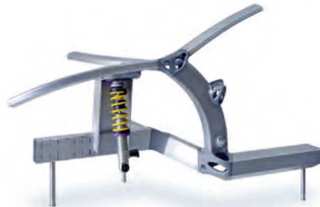
→ Fig.: Next Generation Spaceframe 2.0 – flexible front section structure in hybrid design (source: EDAG)
